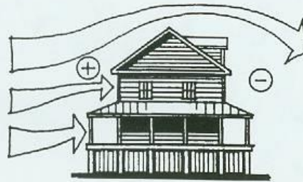
Figure 20: Orienting your home with prevailing breezes compliments the stack effect. The principle of "in low, out high" should be observed.
