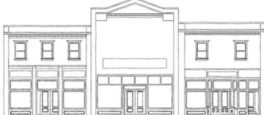
Not Acceptable- Taller gabled parapet and lack of second floor windows
