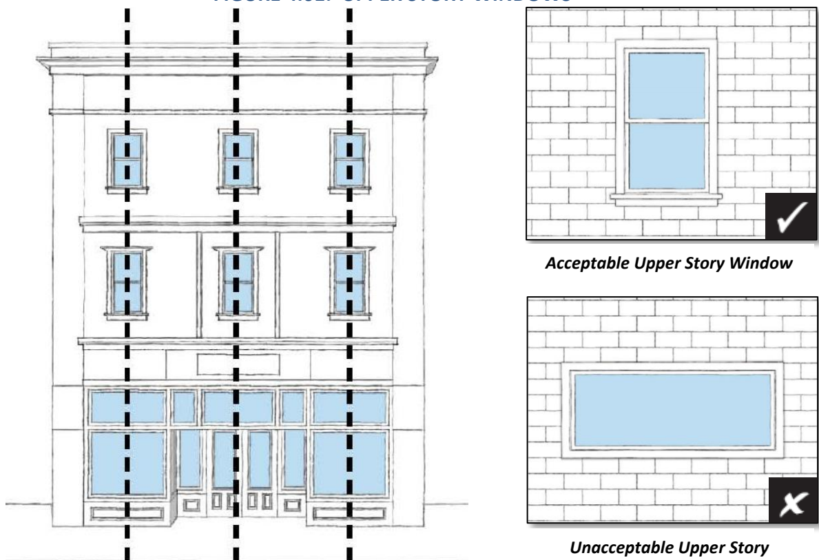
FIGURE 4.61: UPPER STORY WINDOWS
