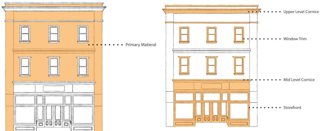
The illustrations above depict appropriate primary (left) and secondary (right) material locations on an example building.
