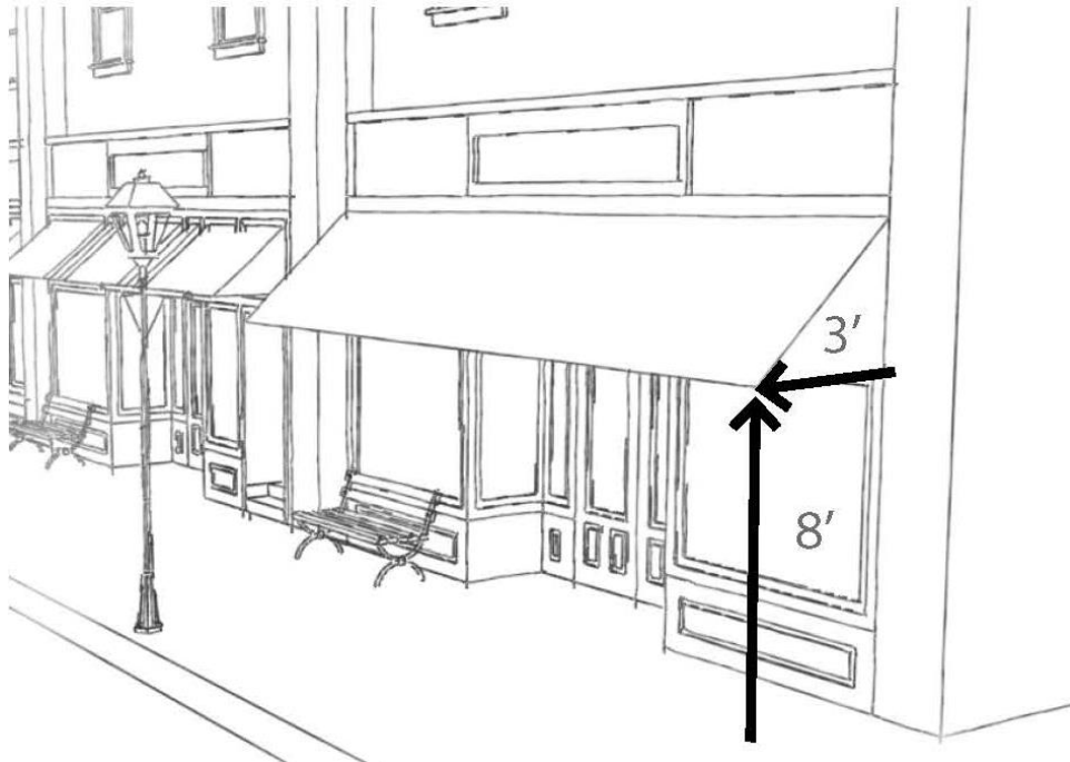
The diagram above illustrates the minimum awning depth and clearance.
