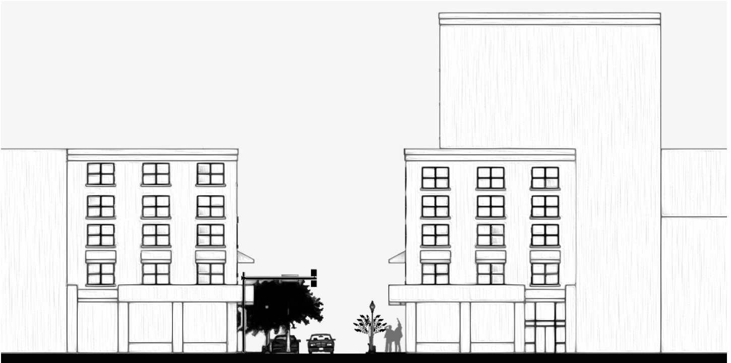
Figure 3.11: Standard Street Section (50' ROW)
