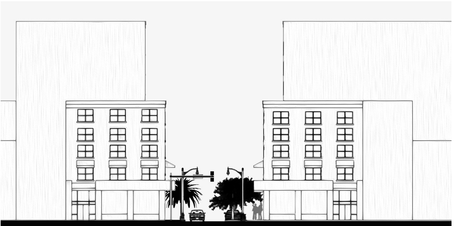
Figure 3.7: Core Street Section (50' ROW)
