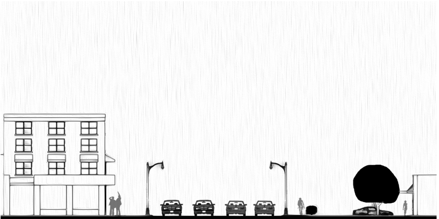
Figure 3.15: Thoroughfare Section (100' ROW)
