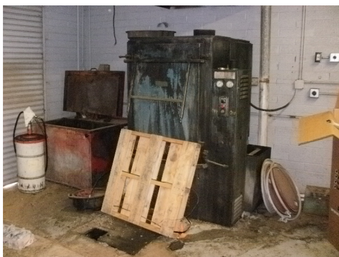
Large parts washer systems adjacent to sump. Note floor staining. Both washers appeared to be dry
