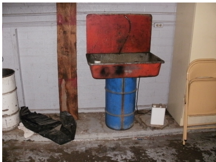
Parts cleaner in automotive repair area. Drum is full of unknown cleaning fluid
